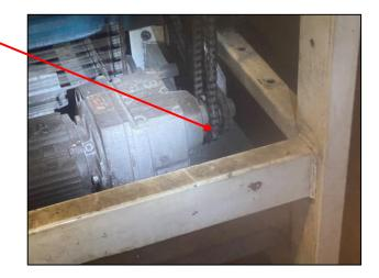
Flour Room – Morning Goods White Sieve Infeed Rotary Valve The motor cooling fan is not turning. It needs re-securing to the motor shaft.
