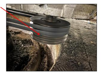
Morning Goods – Prover Raise Gearmotor (Side nearest to BP1) The brake is very noisy when energising. This may be due to a worn brake disk / excessive brake gap. Check / adjust the brake gap.
